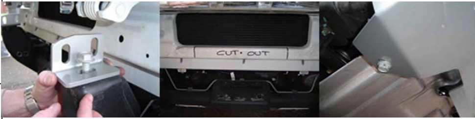
Install Dakar frame mount brackets as shown Inner grill cut out for winch clearance, see drawing below for details Underside bolt location through bumper skid plate
