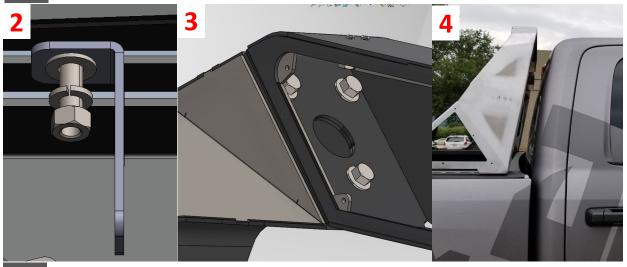
Mark the locations for the 3/4" holes to be drilled (3 per side). Move the headache rack away from the hole location
