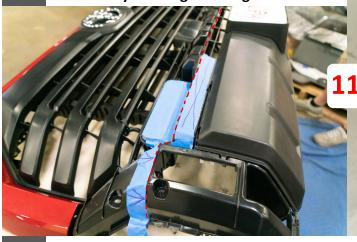
12 Tape along the body lines that are going to 13 Reassemble Grille and Reinstall back onto be cut (Black Dashed Line). truck
