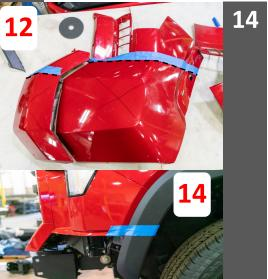
Tape off area of Fender to be cut, lining up with the profile of the previously cut bumper sections.
