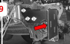
Insert (3) retainer washer per side over a bolt tab inserted through the bumpers slotted holes. You can use a socket to assist in affixing the retainer washers. Measure side to side from the corresponding slots on the frame bracket and position the now "retained" bolt tabs at that same width. This makes it easier to fit up the bumper initially. Once on, align the bumper side to side and tighten bolts.
