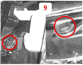
Carefully pry lose. This piece just snaps in place and will be attached to the new bracket provided.
