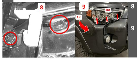
Remove four plastic clips from bottom inside of grille. (One on each side and one in the middle).
