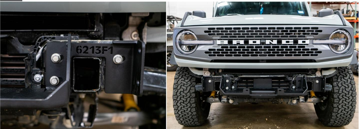
**6** Insert Sensor Housings and Double Nut Plates. Run Wiring Harness and clip Sensors in. Install Lights and Logo. If Equipped, Install ACM into Winch Mount Bracket.
