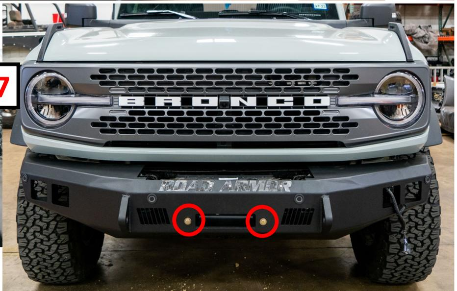
**8** Adjust Fitment of Bumper and Tighten All Nuts and Bolts.
