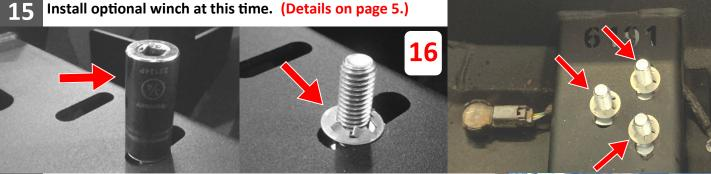
Install 6 - 2" bolt tabs through bumper using the included keeper 16 washers. Use a 3/4" deep socket to push the washers over the threads.
