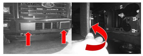
2 Disconnect Lights and Remove Wiring from Bumper.
