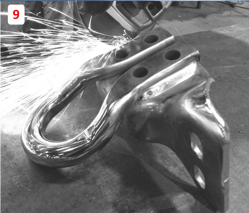
**9** Cut welds to separate the tow hook from the OE bracket
