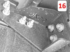
15 Install one single bolt tab per side using included retainer clip by pushing on with a deep socket while holding the back.
