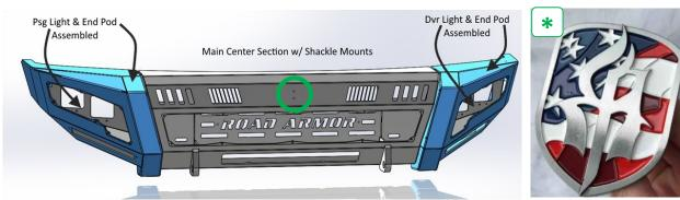
Install Kit Main Center Section "Logo Plate" using Qty: 2 - #10-24x 1/2" Bolts & Lock Nut.
