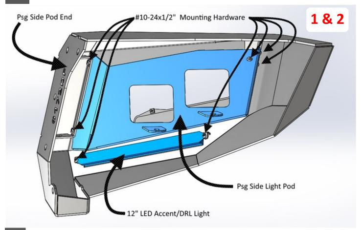
Align and install each kit pod end using Qty:  $6 - 7/16^{\circ}x \cdot 1\frac{1}{2}^{\circ}$  bolts, nuts, lock washers and washers.
