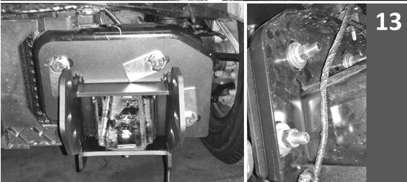
**13** Install brackets using five (5) bolt tabs, followed by a washer, lock washer and nut. Do not tighten bolts fully, or you won't be able to adjust the bumper's fitment and will have difficulty aligning brackets to bumper.
