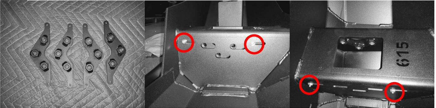
**15** Measure left to right on bumper and adjust brackets to the same distance before attempting fit up.
