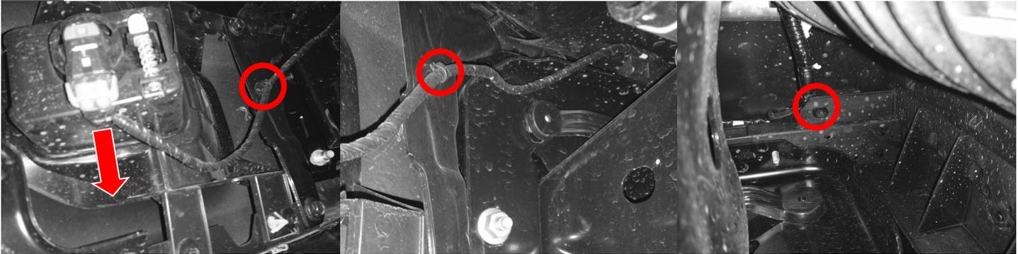
**3** Remove nut on backside of factory bumper on both sides.
