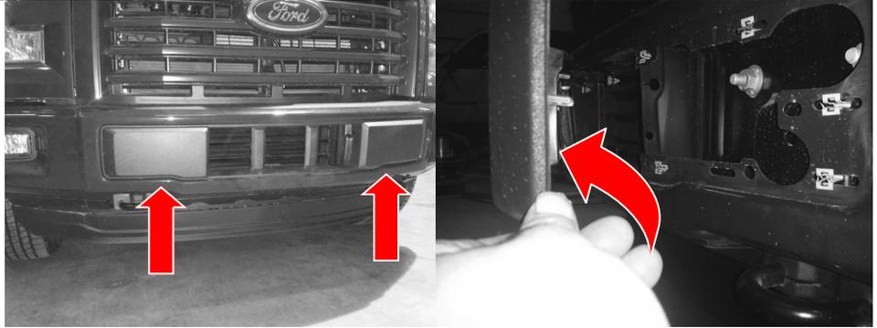
**2** Disconnect Lights and Remove Wiring from Bumper.
