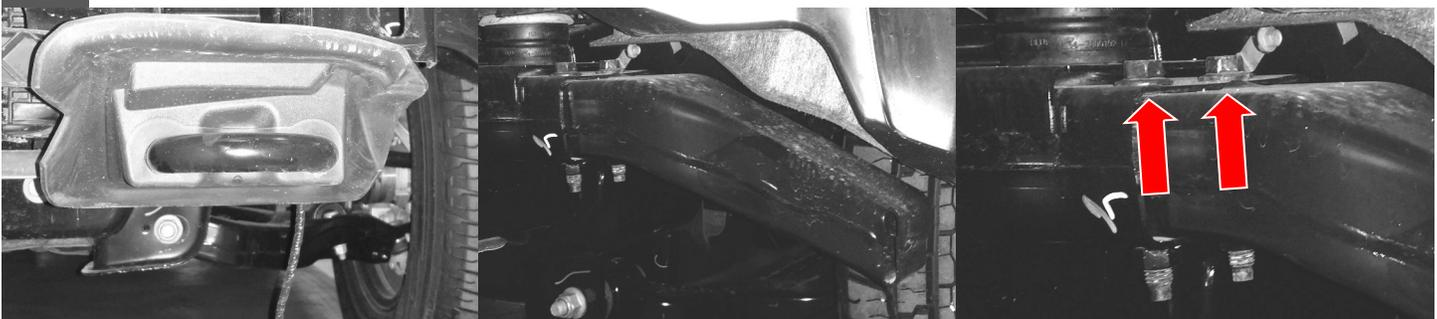
**8** One at a time, thread the included silver flanged head bolt through the nut at the bottom to press the long frame extension bolt up against body to keep it from moving or spinning.
