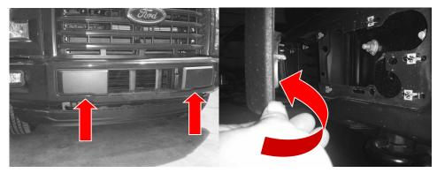
2 Disconnect Lights and Remove Wiring from Bumper.
