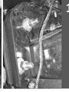
Install brackets using five (5) bolt tabs, followed by a washer, lock washer and nut. Do not tighten bolts fully, or you won't be able to adjust the bumper's fitment and will have difficulty aligning brackets to bumper.
