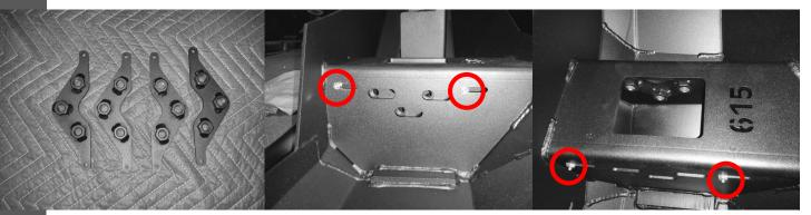
15 Measure left to right on bumper and adjust brackets to the same distance before attempting fit up.
