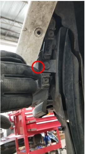
1/2" bolt tabs (2 lower and 2 sides facing inward). Tighten the first bracket to the frame when aligned with second bracket.
