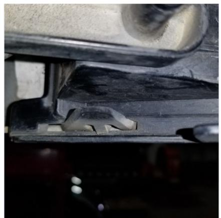
Bolt on the first piece of the brackets using the factory hardware for the top 2 holes and a 1/2" bolt tab for the lower. These will need to be loose enough to allow movement.
