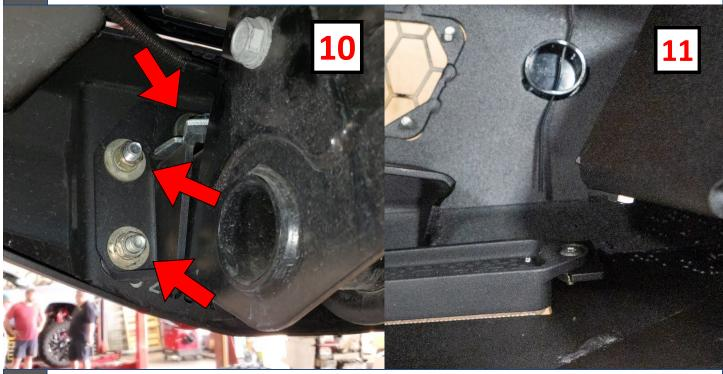
1) Install Side Step/Rock Slider by using the top 2 Factory Bolts (Red) and the Provided 4 inch long Bolt (Green)
