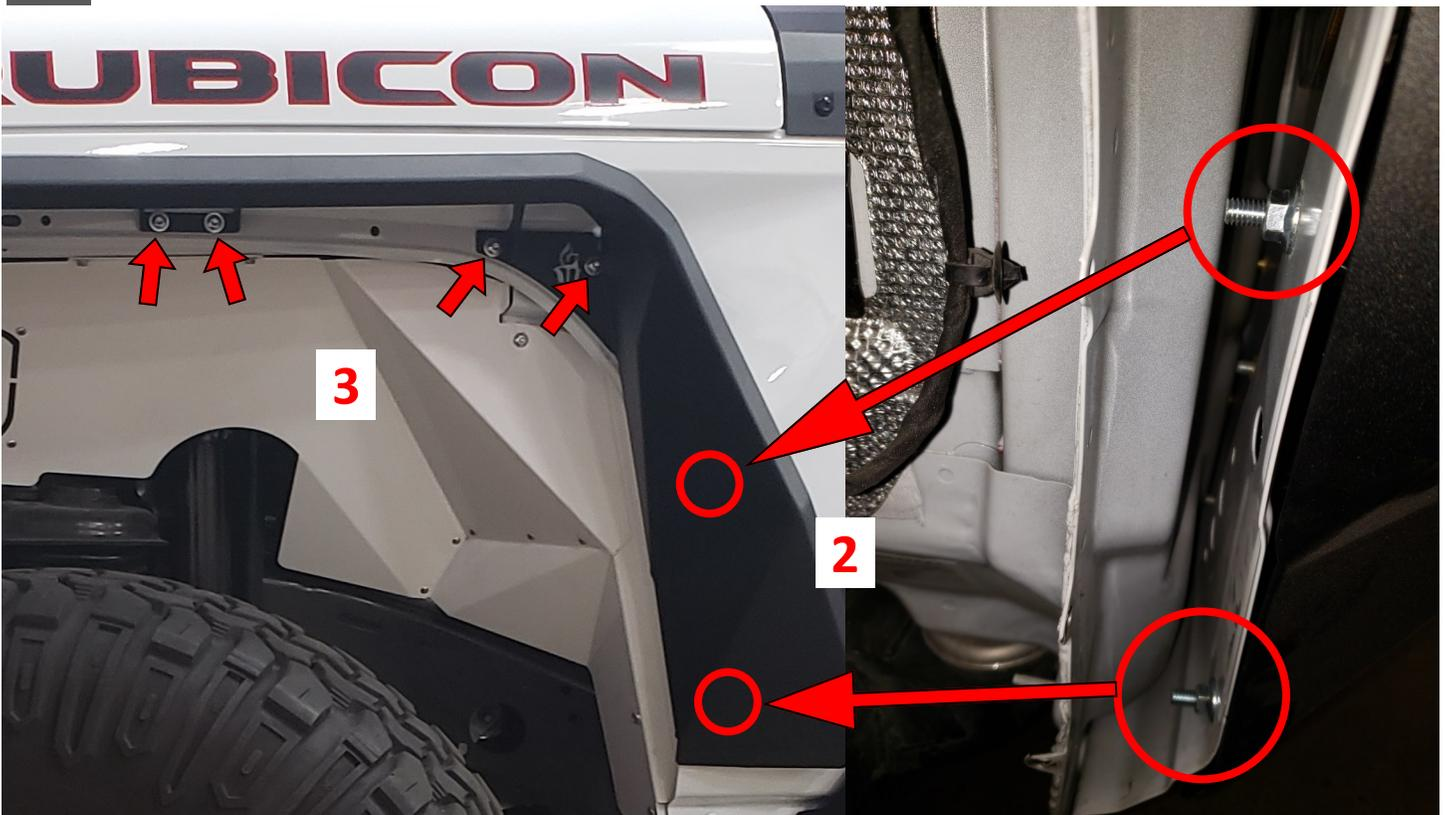
**1** Continue installing FENDER FLARES using 2 - 5/16" HARDWARE as shown below and \*TIGHTEN ALL\*
