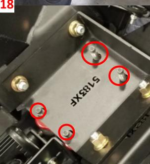
Using the factory nuts, secure the bumper onto the Jeep. Wire lighting options.
