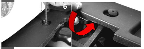
**Remove plastic covering on each side of the bumper using the torx bits and sockets.**
