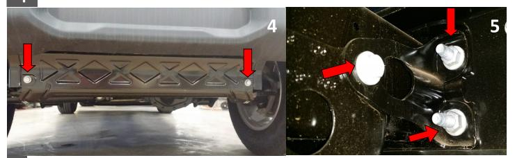
Remove the two nuts one bolt holding the factory bumper and stiffeners on, four (4) on each side of the frame using an 18mm socket and/or wrench. Keep ALL stiffeners for installing Road Armor Bumper.
