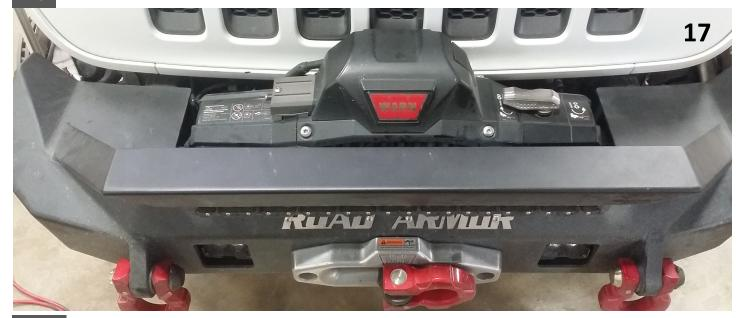
17 If you have a winch to install, do that at this time. (Be sure all wires are secured.) Finished!
