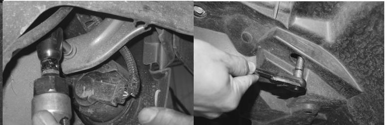
**3** Remove all plastic retainers with removal tool if you own one, or carefully with a pair of dykes or a thin pry bar. Alternatively, just grab and pull the whole inner fender well.
