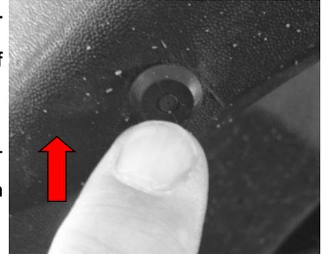
**2** Remove six (6) 10mm Bolts inside fender well and all plastic fasteners. Keep all bolts for future use.
