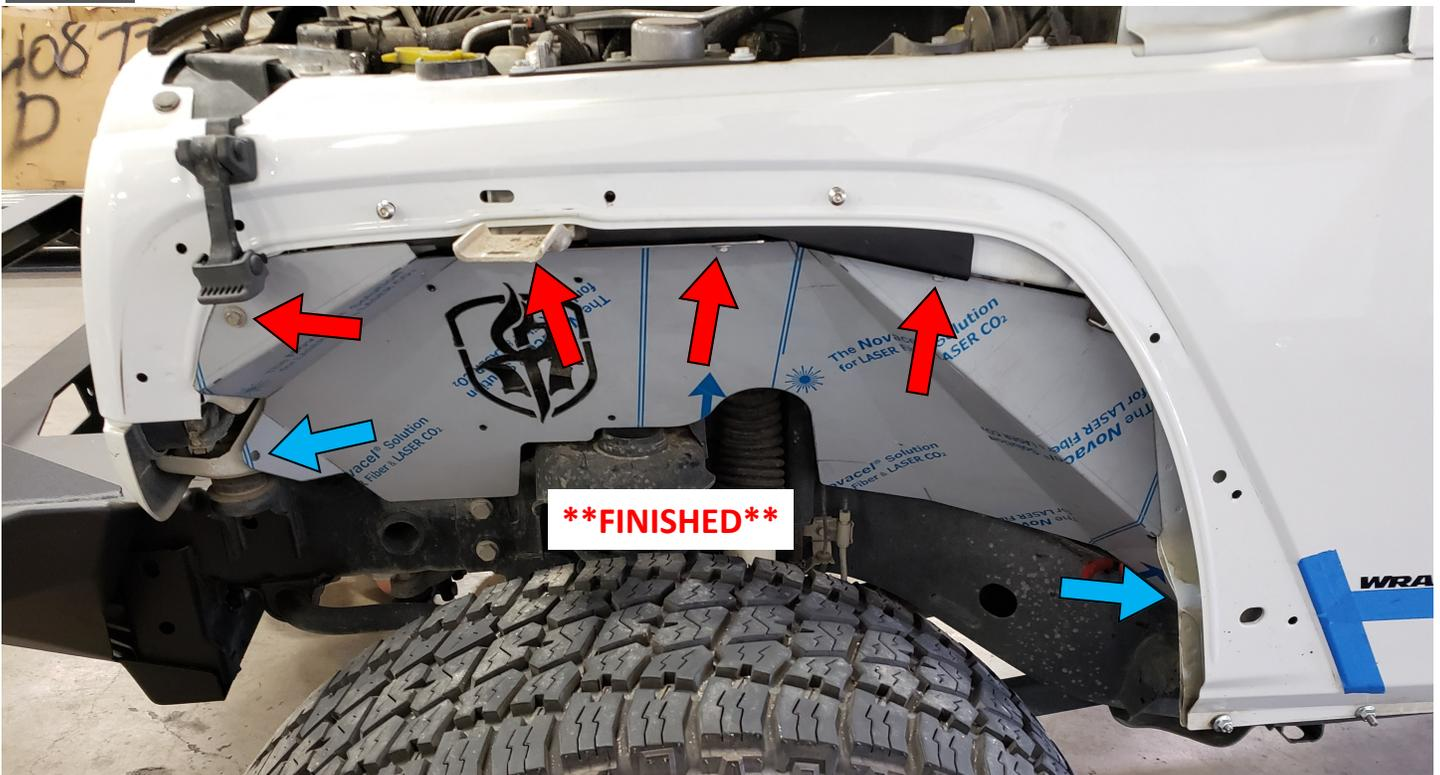
**\*\*Remove protective film after fenders are installed.\*\***
