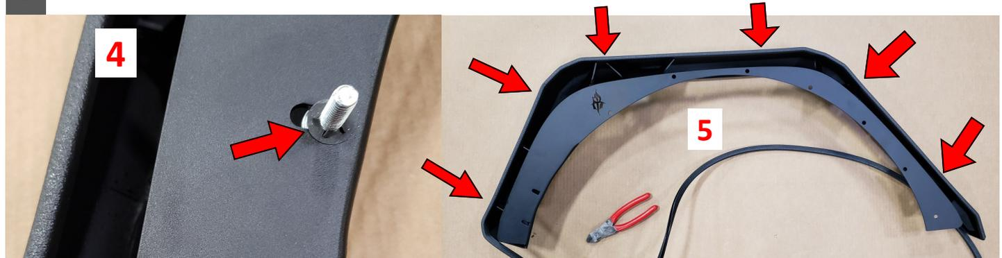
**6** Install REAR FENDER FLARE by inserting both REAR CARRIAGE BOLTS into lower rear holes first. (BLUE Arrow)
