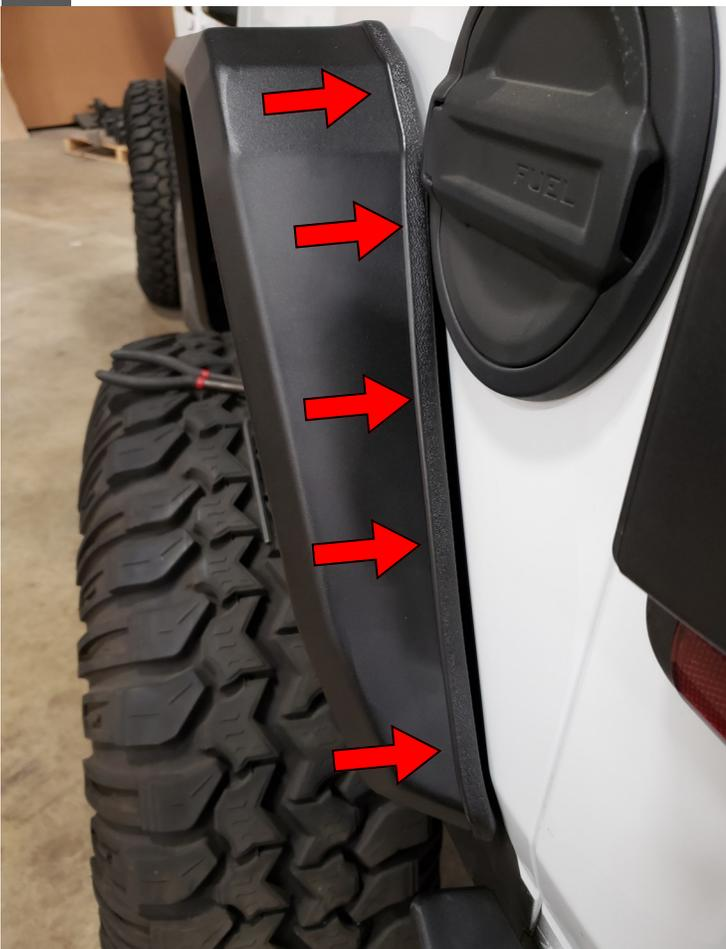
**13** Install modified OE Fender Liners at this time
