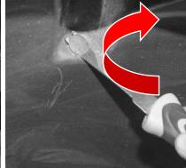
Remove Factory Flare by pulling sharply from the front corner by the grill upward and outward.
