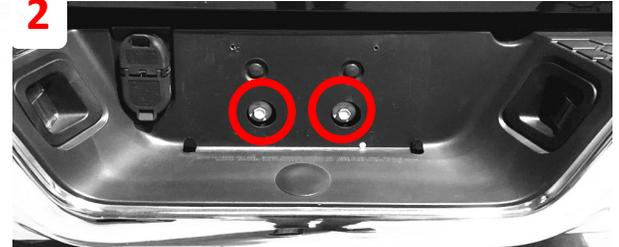
**3** Remove the two bolts from the center of the bumper
