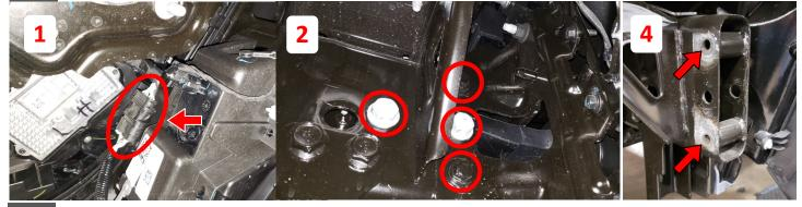
Loosen two bolt securing each intercooler bracket to inside of frame. (Do not remove from frame)
