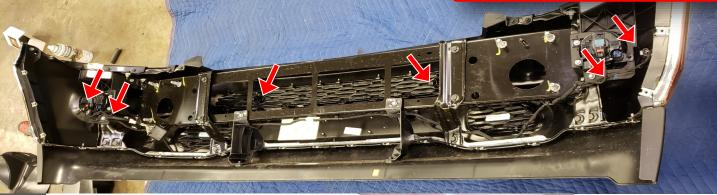
Trim 1/16" off sensor housing for proper fit onto bumper. Zip tie can be used on backside to secure each sensor assembly to bumper for additional security.
