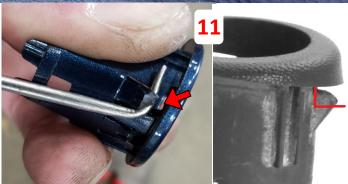
Insert the Single Bolt Tab through outside top slot as indicated, then affix to the bumper side bracket using a retainer clip. Then do the same with the Single Bolt Tab on the opposite side.
