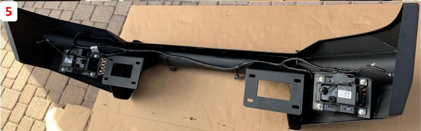
**Note:** Be gentle removing parking sensors. These are easily damaged if subjected to a sudden impact. To remove the sensors, from the rear use a pick tool and slightly pry the housing away from the tabs on the sensor. Push on the front of the sensor and it will slide out the back.
