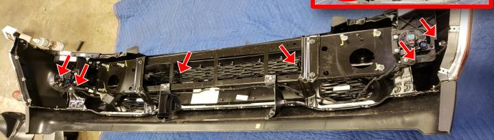
Trim 1/16" off sensor housing for proper fit onto bumper. Zip tie can be used on backside to secure each sensor assembly to bumper for additional security.
