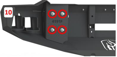
Install the winch to the bumper using the supplied Allen Bolts and Washers.
