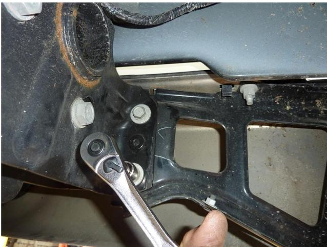
**NOTE: Bumper will be removed during this step. Be prepared to hold bumper in place and remove once bolt plates are removed.**
