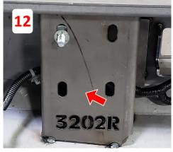
\*NOTE: DVR Side Hitch Tube May Need 1/4" Material Removed From End Of Hitch Tube To Provide Clearance For Support Bracket To Sit Flush On Mounting Bracket.\*
