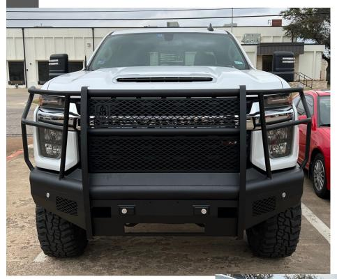
\*MINIMUM 3/8"+ Gap Required; DO NOT Install Directly Against Front Facia\*
