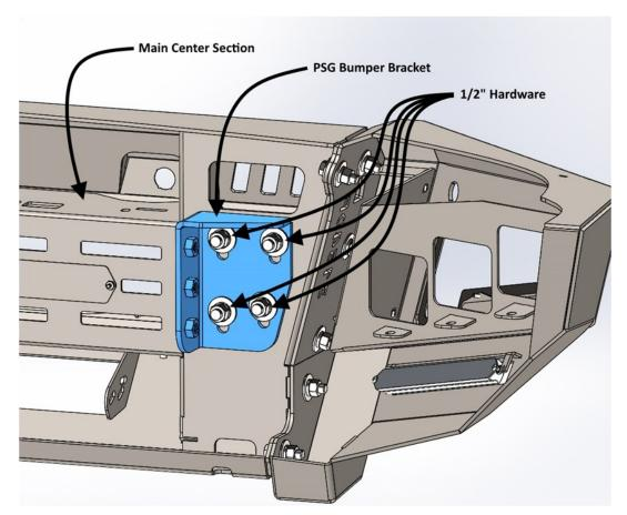
\*\*NOTE: Be sure to install grille assembly prior to installation of iD front bumper. Doing so will allow proper alignment of bumper profile to truck when installing bumper.\*\*
