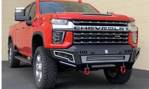
\*\*NOTE: Be sure to install grille assembly prior to installation of iD front bumper. Doing so will allow proper alignment of bumper profile to truck when installing bumper.\*\*
