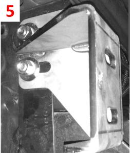
Install bumper brackets onto the frame using supplied hardware
