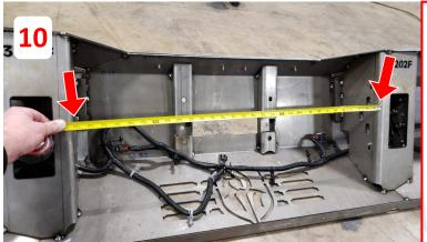
\*MINIMUM 3/8"+ Gap Required; DO NOT Install
