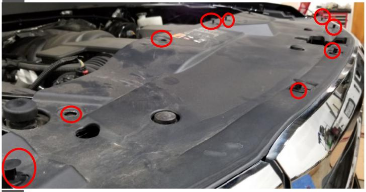
2 Remove the top 4 bolt securing the grill.
