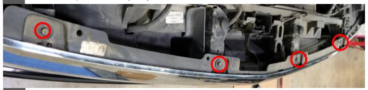
Remove bolts the lower bolt in the inner fender liner.
