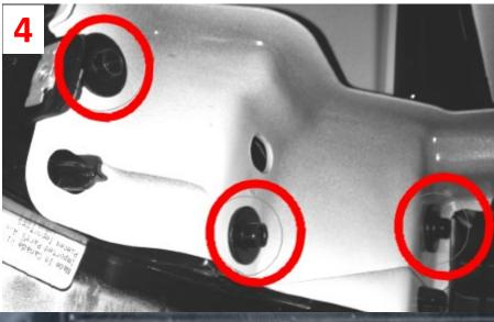
5 Remove the 4 bolts holding the lower grill in place.
