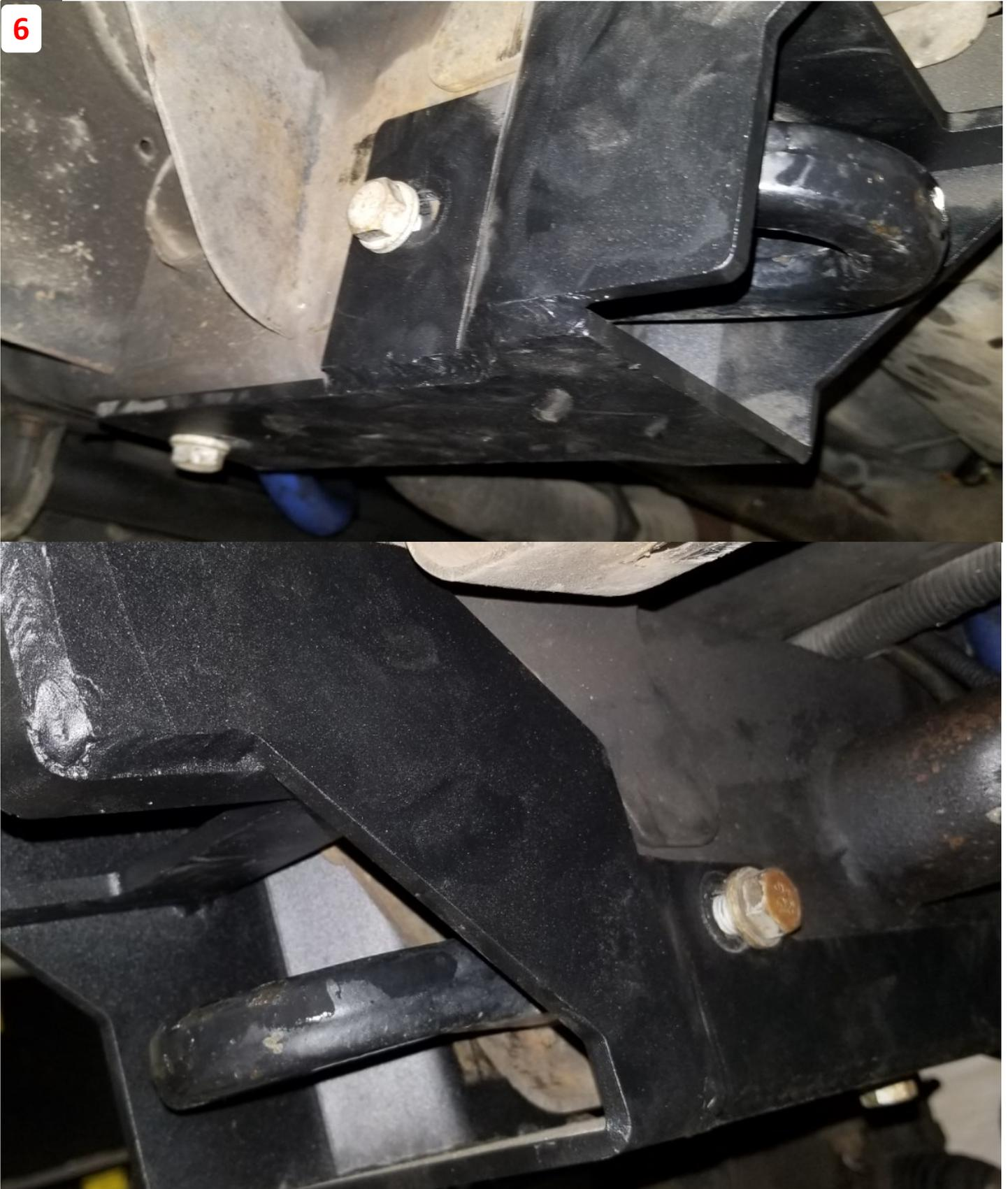
**7** Install the small of the 2 brackets onto the top of the frame using factory hardware.
