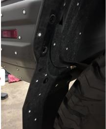
Once End Pods are Removed, Unbolt the Bracket that was supporting the End Pod.
